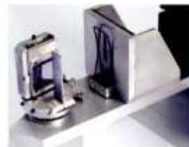
Curved graphite crystal monochromator
