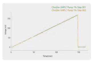
⟨Ultra fast gradient response for precision of solvent composition⟩
